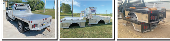
Pictures of the Hillsboro 500 and 1000 series Hybrid Flatbed, Steel flatbed fully skirted in aluminum with tool boxes.
